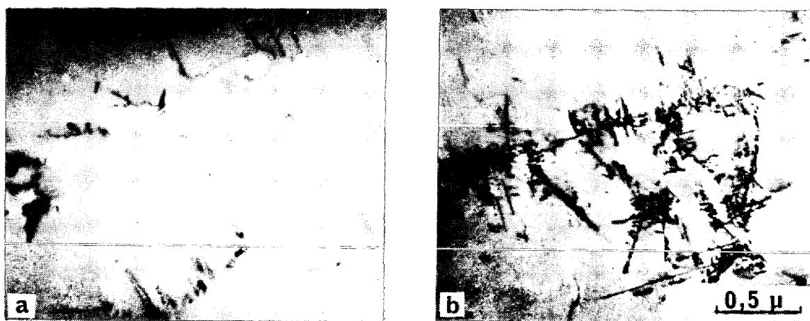
Photo. 5. Transmission electron micrographs of nucleation and growth of M_{23}C_6 carbides within grain of H42A aged at 700^\circ\text{C} .
