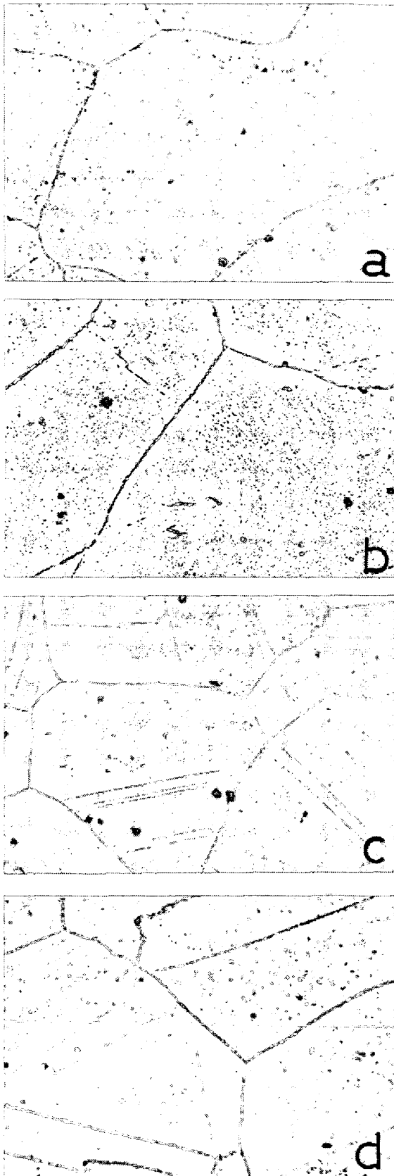
Photo. 4. Microstructures of specimens cold rolled by (a) 0%, (b) 5%, (c) 7.5%, (d) 9% and subsequently annealed at 1000°C for 150h ( \times 200 ).
