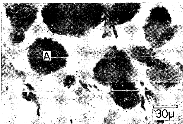
Photo. 2. SN-8 synthetic slag after dipping into water for 5 sec. [A] homogeneously hydrated free lime.
