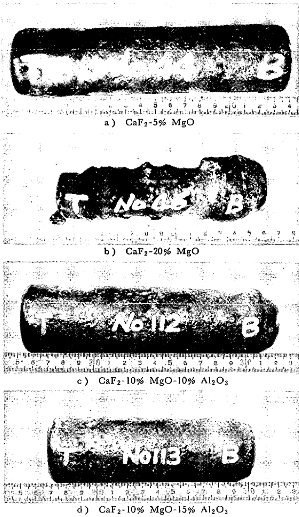
Photo. 2. Surface appearance of ESR ingots remelted by \text{CaF}_2 -MgO and \text{CaF}_2 -MgO- \text{Al}_2\text{O}_3 slag.
