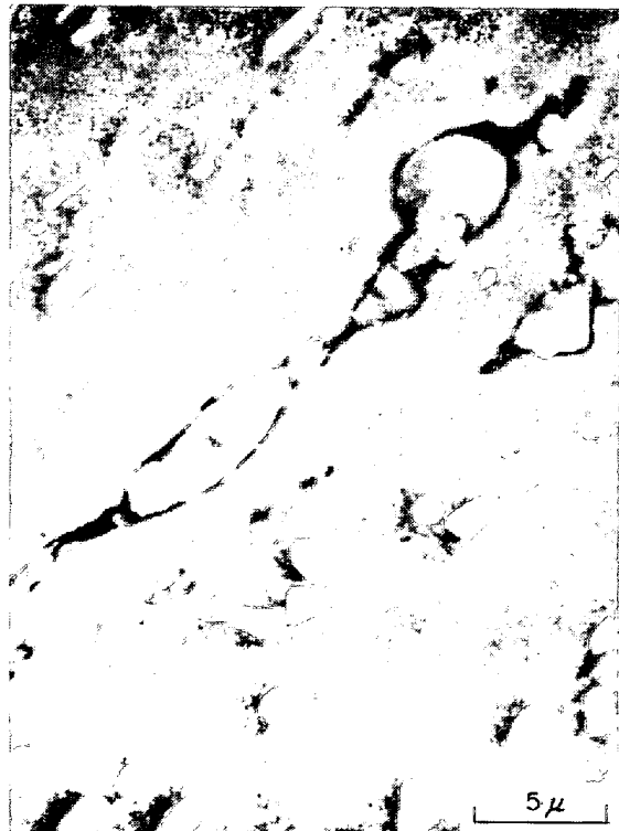
(b) Globular sulphide inclusions in No. II-A-5 steel. Etched with 5% nital.
