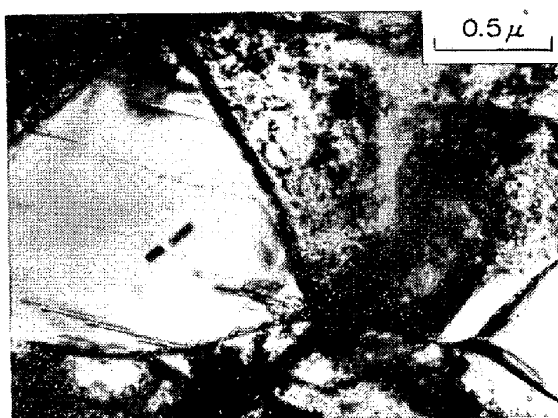
Photo. 6. Dislocation in carbide (cementite) observed in steel A, strained to \epsilon=0.3 .
