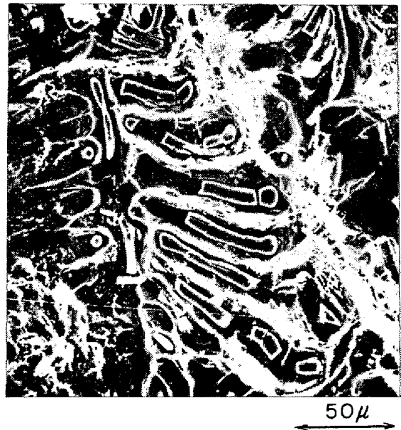
Photo. 4. Fracture surface of Z direction Charpy specimen of slab showing morphology of type II MnS. (reduction 62%)
