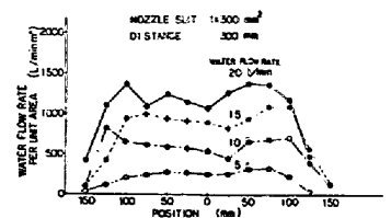
Fig. 3. Profile of water density in the case of a mist-jet nozzle.
