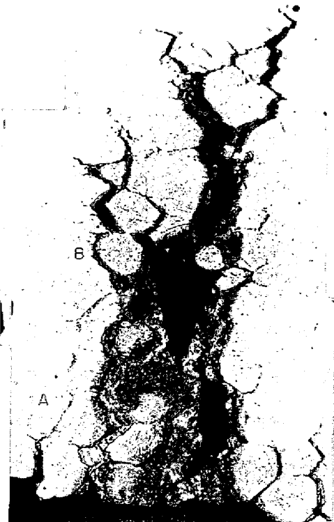
Photo. 1. Crack of SSS410 test piece ruptured in air at 1680 hours, showing a lot of nitrides around crack. (x100)
