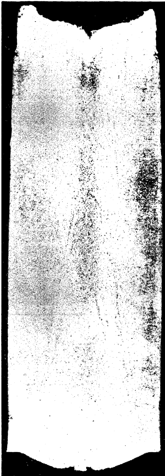
Photo. 1. Macrostructure of 11 t ingot. (x3/4)
