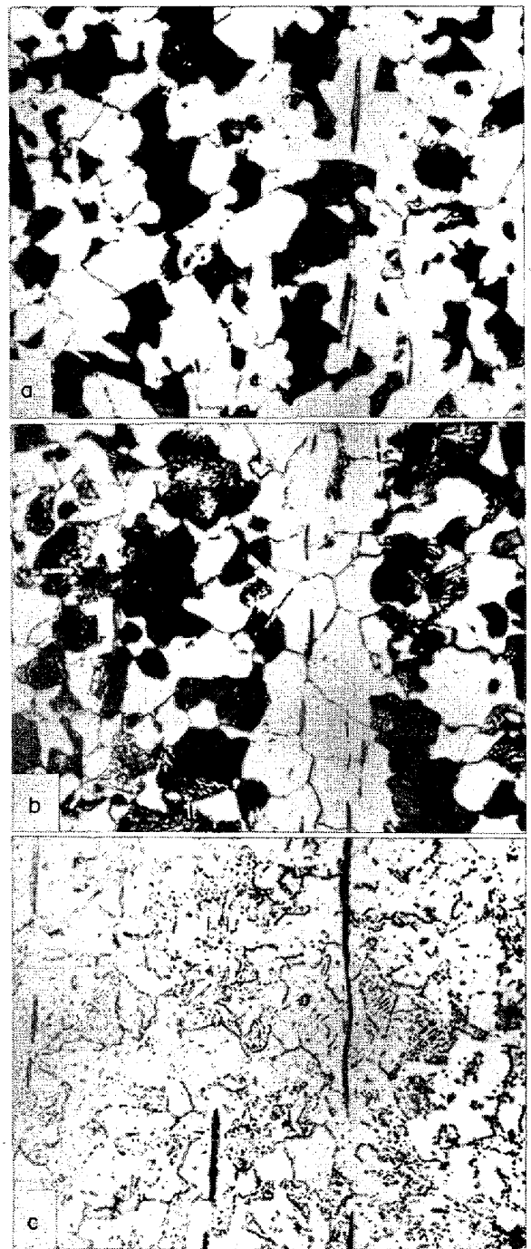
(a) Normalized ( H_B 167) ×400 (b) Annealed ( H_B 154) (c) Spheroidized ( H_B 144)
