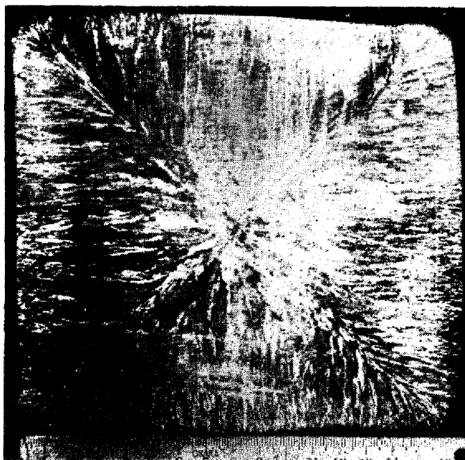
b) Internal cracks, caused by Depression at corner
