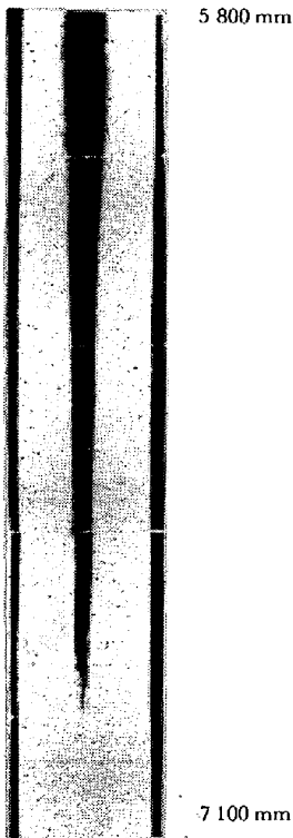
Photo. 2. Autoradiographs showing distribution of Au 198 in test slab E. (×1/15)
