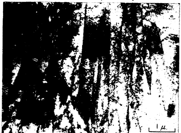
Photo. 7. Electron-microscopic picture of Fe-25.4% Ni-2.17%Mn alloy transformed for 45 minutes at -80^{\circ}\text{C} isothermally. The micro-structure is very like to the lath structure of the so-called packet type athermal martensite.
