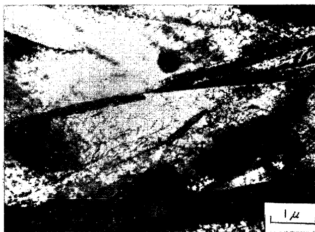
Photo. 17. Micro-structure of the martensite and the austenite in Fe-25.3%Ni-4.52% M_0 alloy transformed at -196^{\circ}\text{C} . The lenticular martensite containing twins and the lath type martensite can be observed. The dislocation density in the austenite is much higher than that in the austenite surrounding martensites transformed isothermally at higher temperature.
