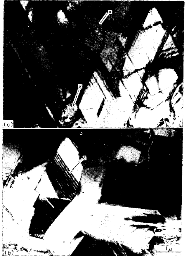
(a) The specimen was cooled after austenitizing at 900^\circ\text{C} for 10 min. Both \gamma \rightarrow \epsilon and \epsilon \rightarrow \alpha transformations took place. (b) The specimen was cooled immediately after reached to austenitizing temperature of 800^\circ\text{C} . Only \gamma \rightarrow \epsilon transformation occurred.
