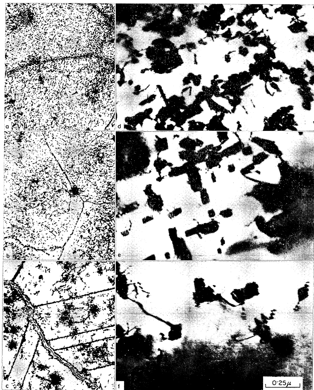
×600 a, d) Water quenching b, e) Air cooling c, f) Furnace cooling
