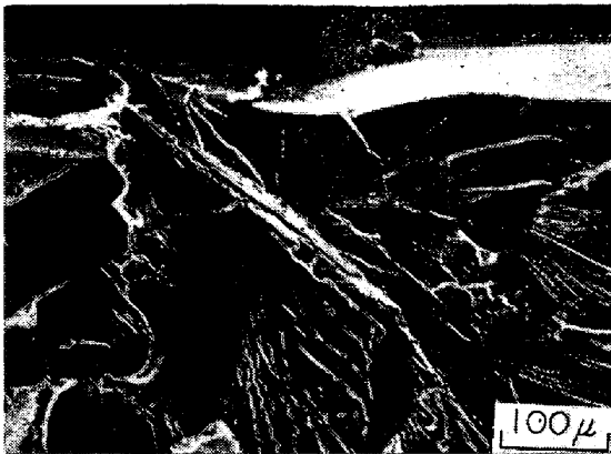
Photo. 4. Fracture initiation from twinning in notch root. Closed circle shows the initiation point of cleavage fracture. Impact (10 m/sec, -105^{\circ}\text{C} )
