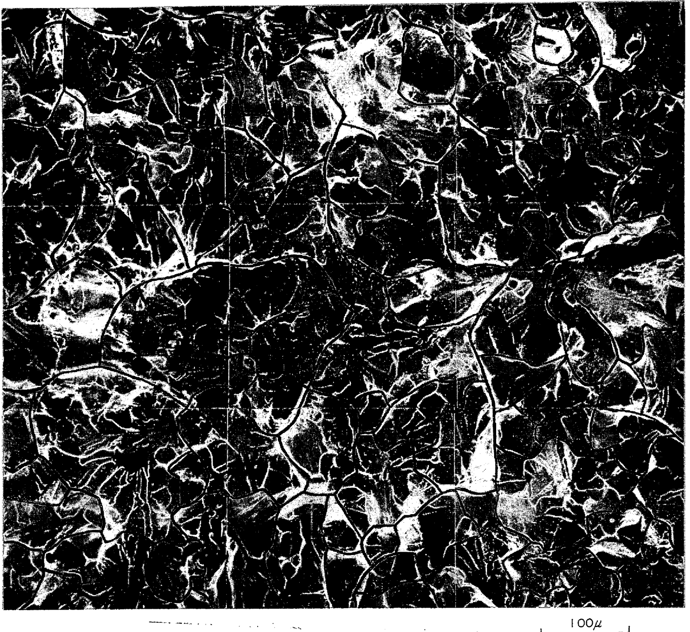
Photo. 4. Typical fracture surface of sample A after Charpy impact test (in Z-direction)
