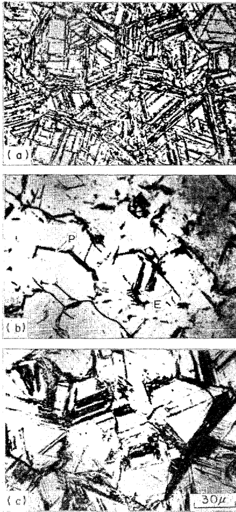
Photo. 4. Effect of pressure on martensite microstructure in Fe-0.28%C alloy (A-2). (a) Packet structure (P), quenched to 230°C at 29kbar. (b) Packet (P) and plate-like (E) structure, quenched to 220°C at 38.5 kbar. (c) Plate-like structure (E), quenched to 180°C at 41kbar.
