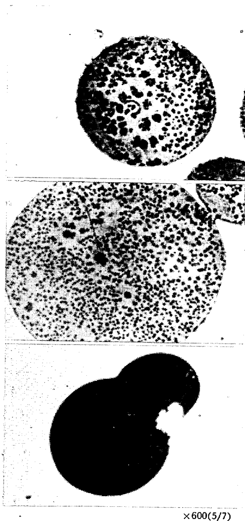
Photo. 5. Coaguration process of oxide particles on the deoxidation with calcium-silicide.
