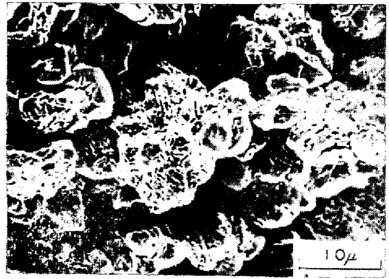
Photo. 6. Magnetite surface structure after partial reduction of \alpha -hematite at 900°C in H 2 -H 2 O mixture (P H 2 = 0.17 atm, P H 2 O = 0.83 atm).
