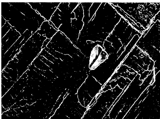
Photo. 6. Two twins, T1 and T8, intersected along [110] direction, however, where no cleavage crack was nucleated. (Stereo viewing)
