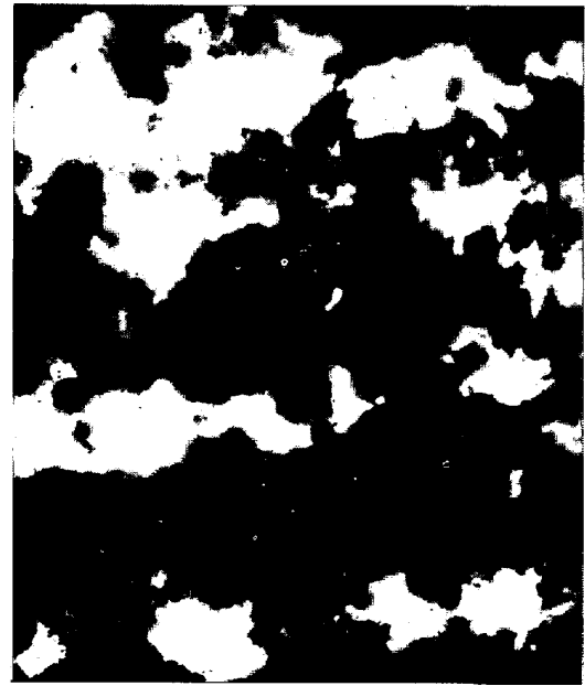
(A) Transverse (B) Longitudinal Photo. 4. Photomicrographs of transverse and longitudinal sections. Same specimen as in Photo. 3. Stead's reagent etched. \times 100 (9/10)
