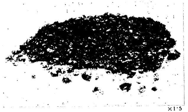
Photo. 3. Appearance of alumina powder collected from surface of ingot with tellurium treatment.
