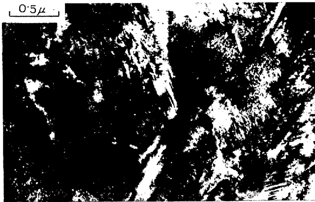
Photo. 1. Transmission electron micrograph of an untempered martensite of 0.48% C steel showing fine twins.
