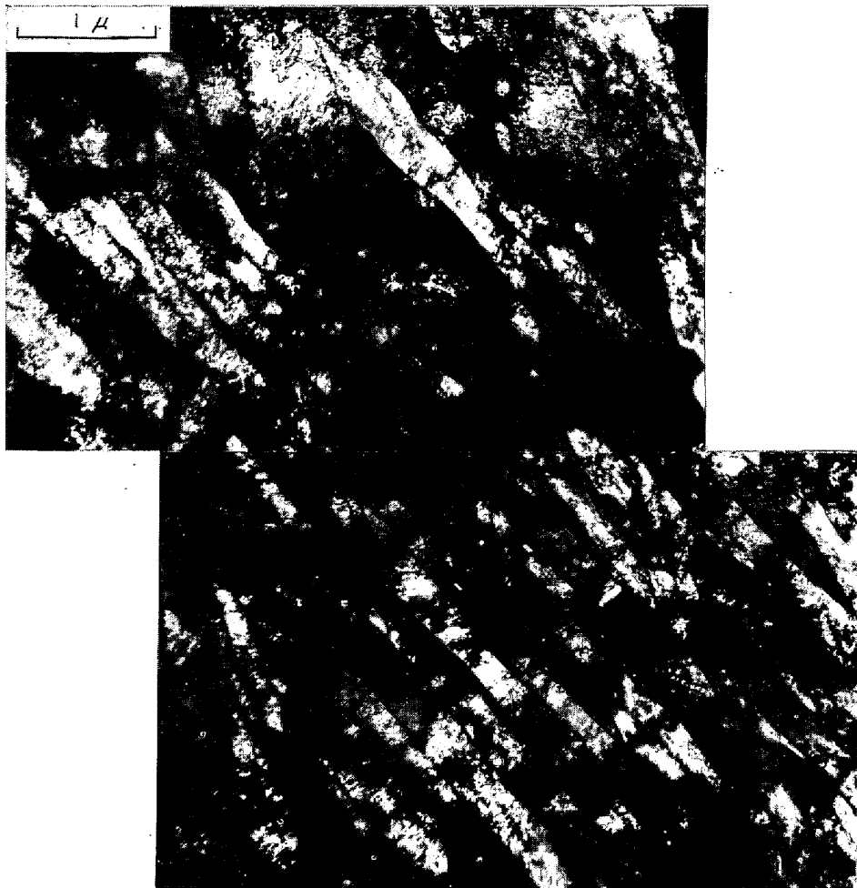
Photo. 10. As quenched structure of 0.017% C steel showing lath martensite.
