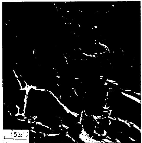
Photo. 11. Microfractograph of grey cast iron tested at -196^{\circ}\text{C} . Cleaved graphite (upper left) and many cleavage type facets are observed.
