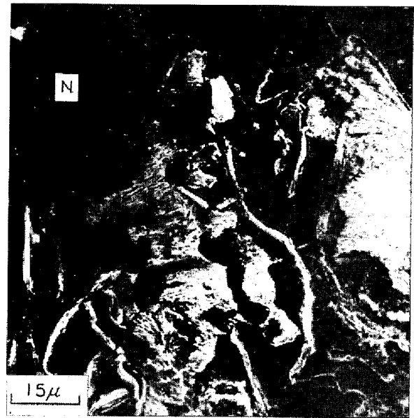
Photo. 7. Fracture profile of grey cast iron tested at -20^{\circ}\text{C} . Main crack avoids to pass through pearlite regions and, in some cases, it passes through along ferrite-pearlite interface (upper right). N : Ni plate
