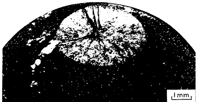
Photo. 2. Fish-eye on the fatigue fracture surface of carbonitrided cast carbon steel (SC37).
