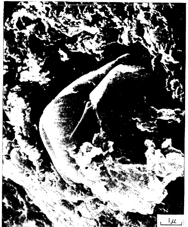
Photo. 4. Non-metallic inclusion at the center of fish-eye on the fatigue fracture surface of carburized carbon steel.
