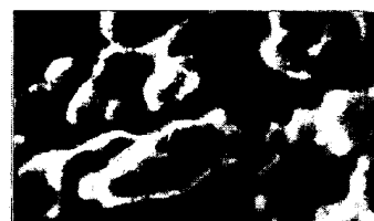
Photo. 3 Reduction at 900^\circ\text{C} Sintered synthetic \text{Fe}_2\text{O}_3 pellets (100% reduced)
