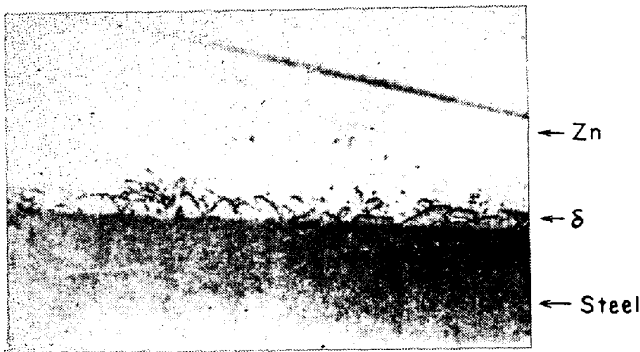
Photo. 4. Microsection of coating with an immersion time of 30 seconds and aluminium content of 0.12% (alloy layer phase : \delta ) \times 1000 (7/9)
