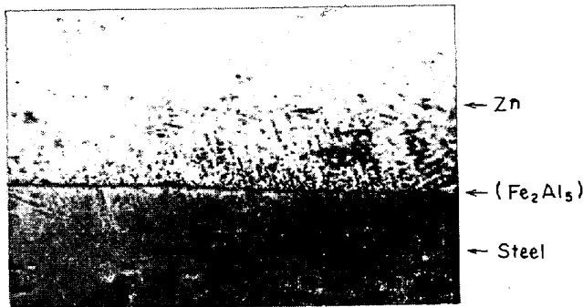
Photo. 5. Microsection of coating with an immersion time of 30 seconds and aluminium content of 0.15% (alloy layer phase : \text{Fe}_2\text{Al}_5 ) \times 1000 (7/9)
