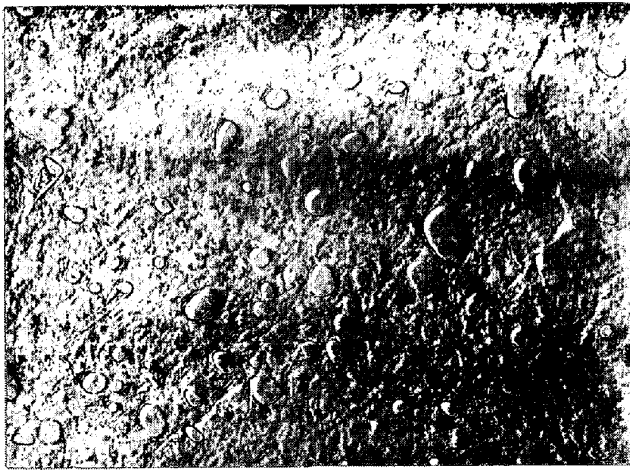
Photo. 1. Electron replica micrograph of the Sk 3 steel spheroidized at 740°C for 4 hr.
