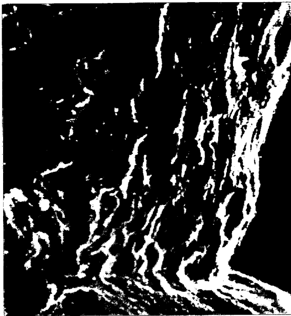
7.5 \times 10^{-6} He Stress 6 \text{ kg/mm}^2 , rupture life 1 hr
