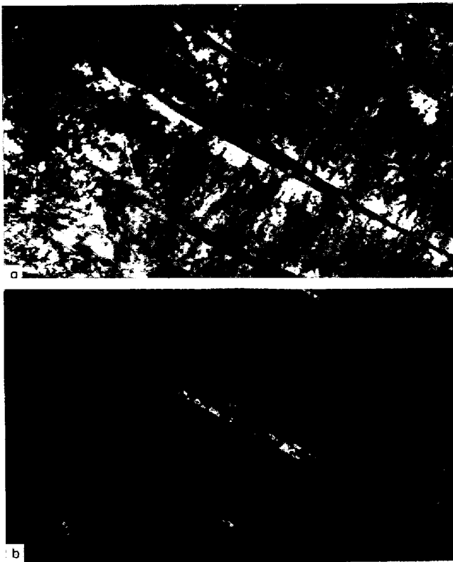
Photo. 3. The bainite I formed at the temperature as low as 475°C (a) the bright field image, and (b) the dark field image using a martensite reflection which arose from the layers between the bainite laths.
