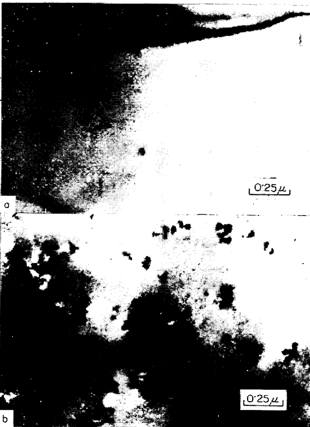
Photo. 7. Transmission electron micrographs of specimens solution-heated at 1200°C, furnace-cooled to (a) 750°C or (b) 700°C, respectively, and then air-cooled.
