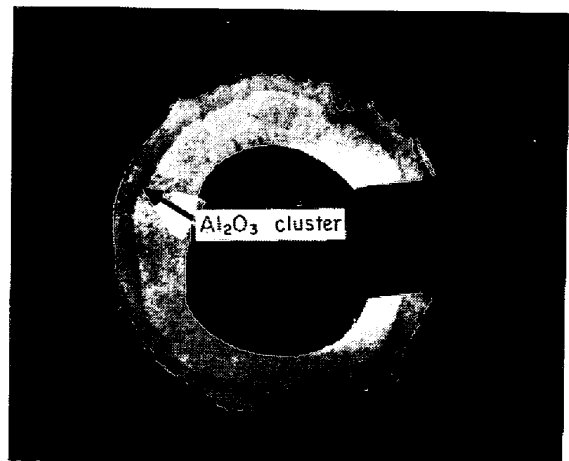
Photo. 2. Cross section of nozzle clogged.
