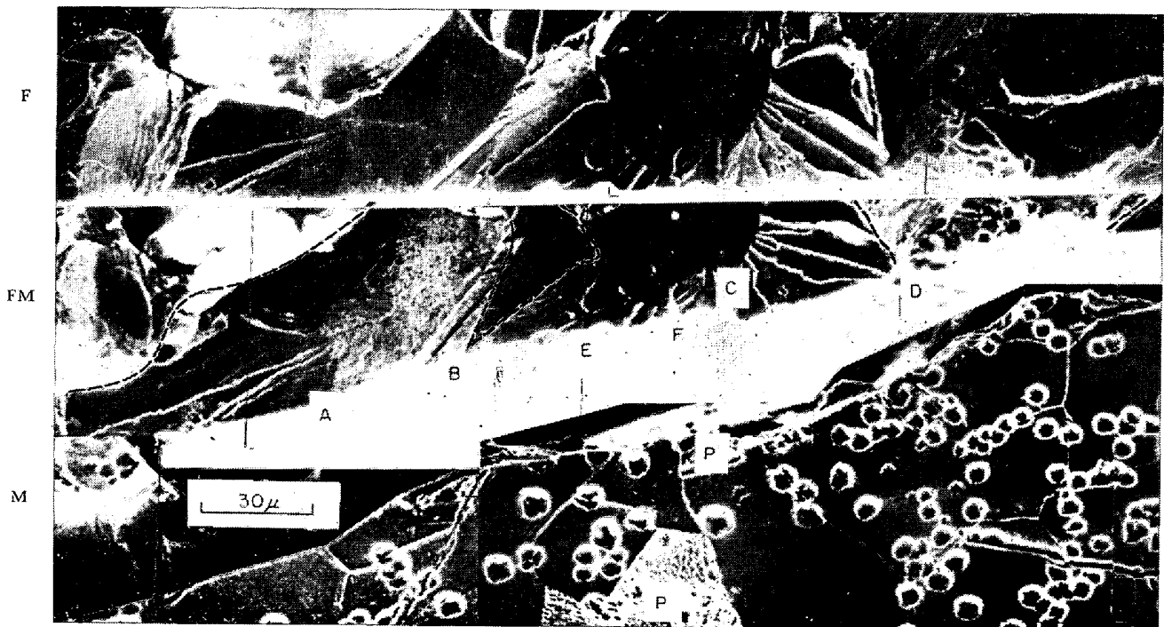
Photo. 3. Direct correspondence between fracture surface and microstructure. (ferrite-pearlite) A~F indicate the grain boundaries and the dotted lines indicate microfracture units. (P: pearlite)
