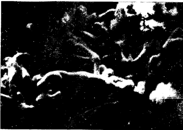
Photo. 4. Metallic iron filament in reduced pellet of Brazil ore.
