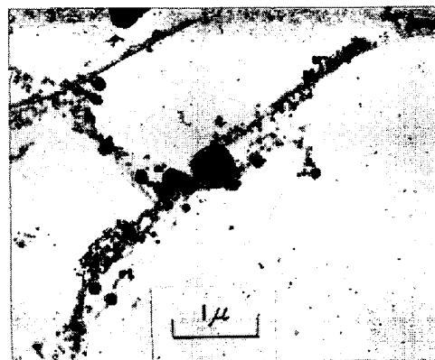
Photo. 3. Electron micrograph of MnTe found in cold-rolled sample B. (extraction carbon replica).
