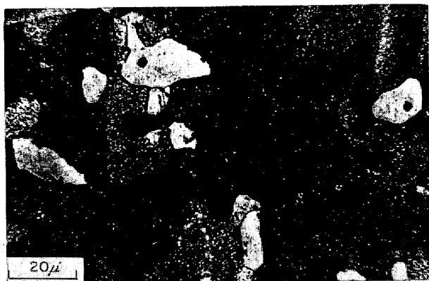
Photo. 6. Optical micrograph of the fine-grain specimen, cold rolled 75% and annealed 30 sec at 500°C.
