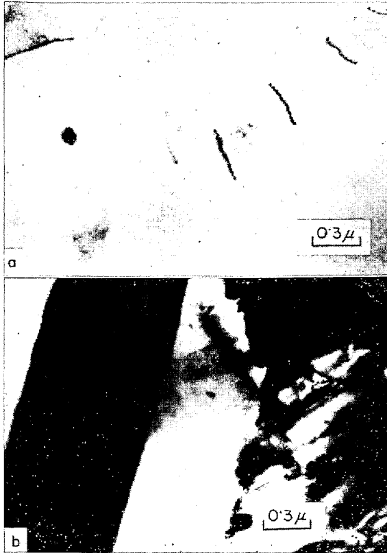
(a) Matrix without grain boundary reaction. (b) Grain boundary reaction and residual carbide.
