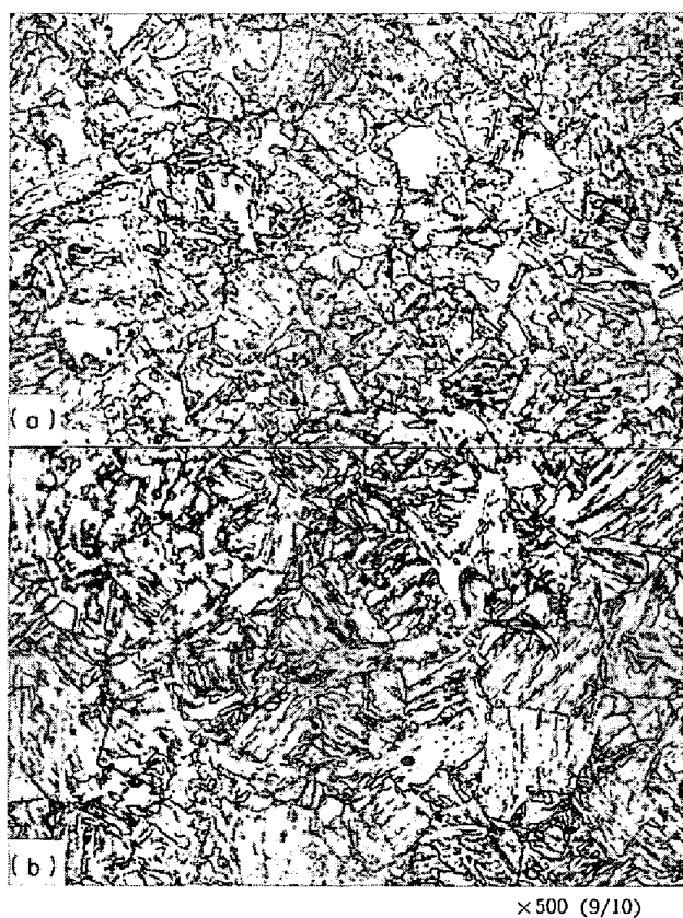
Photo. 1. The optical micrographs of the bainite. (a) The steel E 319 (1%Ni) heat treated in the salt bath held at 350°C for 2 min after austenitizing at 950°C. (b) The steel E 321 (3%Ni) transformed similarly at 350°C for 5 min.
