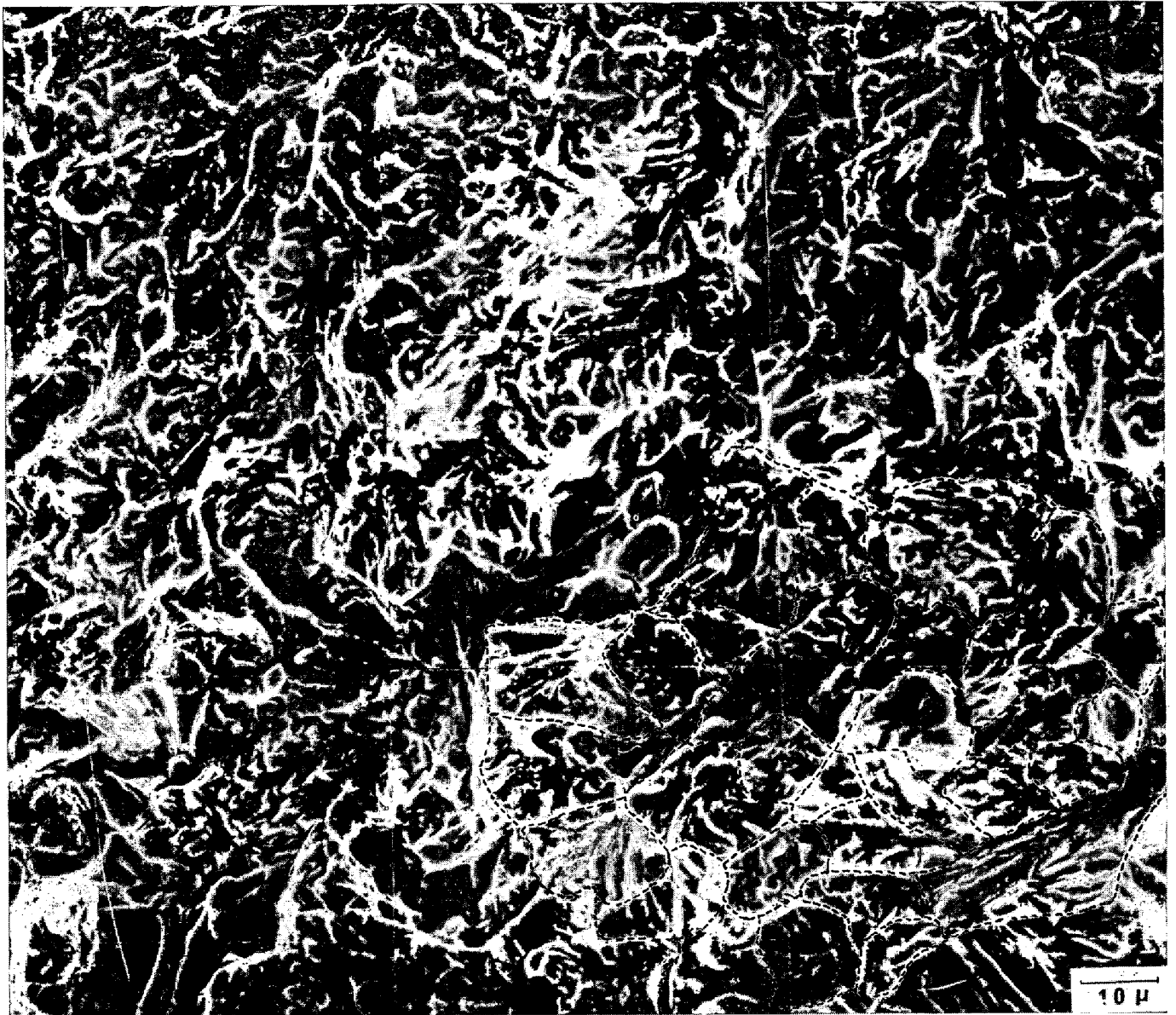
Photo. 12. The brittle fracture surface of the tempered bainite in the steel E 321. (Transformed in the salt bath held at 350°C for 5 min and tempered at 650°C for 1hr, and then fractured at -196°C.)
