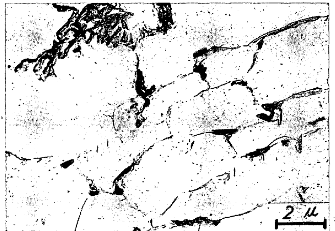
Photo. 4. Electron micrograph showing cementite morphology produced in type II transformation in Nb steel deformed at 800°C.
