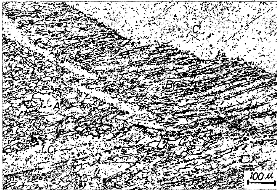
A : recrystallized austenite grains B : deformation band in nonrecrystallized austenite grain C : nonrecrystallized austenite grain
