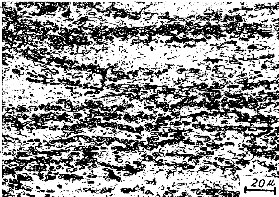
Photo. 2. Fine ferrite grains transformed immediately after hot working at 800°C in Nb steel, etched with saturated picric acid containing sodium benzen sulfonate.
