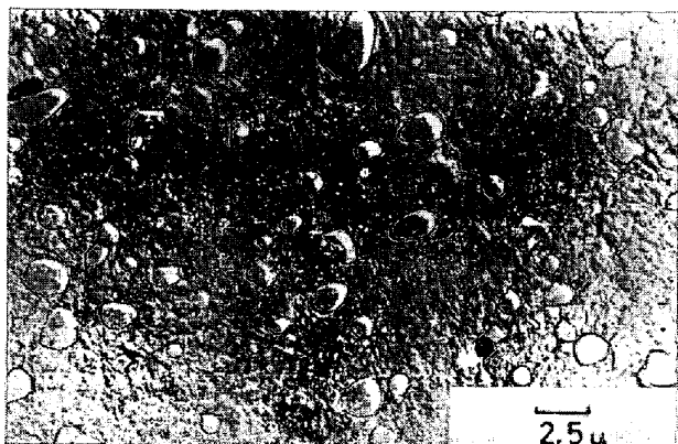
Photo. 6. Electron micrograph of carbide structure in powder forged steel, JIS SKH-2.
