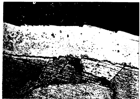
Photo. 4. Micro-structures of boundary between chromized layers and substrate for high carbon austenitic steel.
