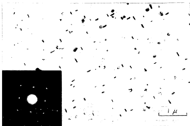
Photo. 1. Electron micrograph and electron diffraction pattern of carbon extraction replica of TiN in Fe-0.1% Ti alloy internally nitrified at 700°C × 4 hr and annealed at 850°C × 48 hr.
