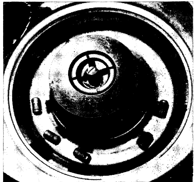
Photo. 1. Position of the graphite capsule in the heating zone of vacuum furnace.
