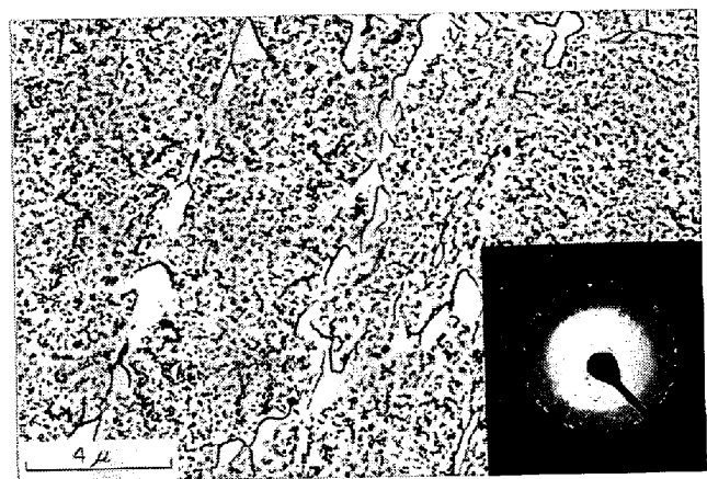
Photo. 6. Electron micrograph of Fe-18%Ni-3%Si alloy aged for 100hr at 500°C. (Extraction replica)
