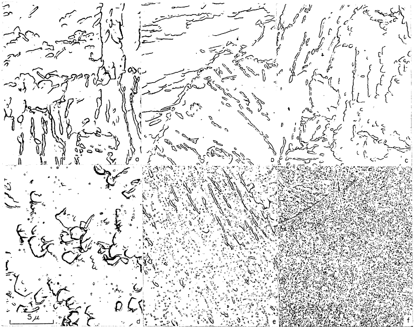
Photo. 8. Microstructures of Fe-15%Ni-Si alloys aged for 500hr at 475°C. (a) 0.005%Si, (b) 0.45% Si, (c) 0.94%Si, (d) 1.45%Si, (e) 1.99%Si, (f) 2.93%Si.
