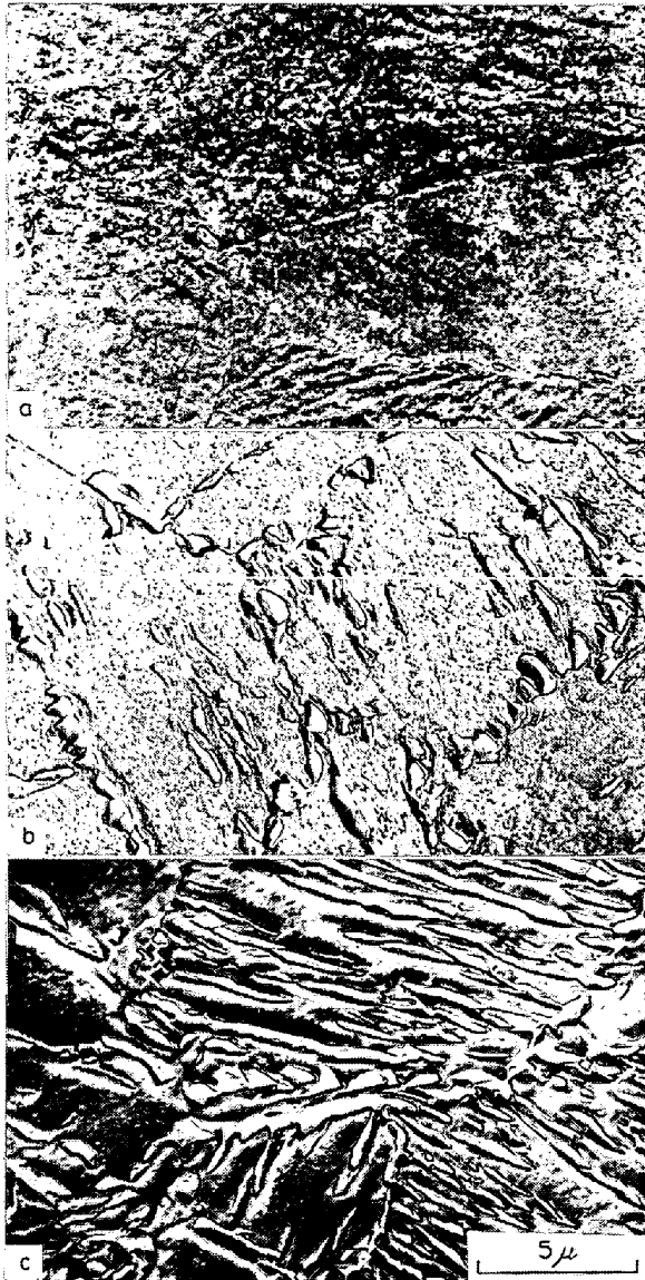
Photo. 1. Microstructures of Fe-18%Ni-3%Si alloy solution treated at 1000°C and aged for (a) 5hr, (b) 100hr at 500°C, and (c) 3hr at 575°C.
