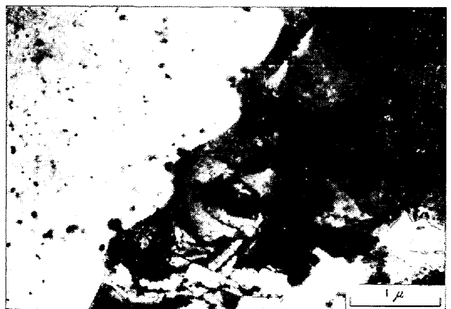
Photo. 6. Electron transmission micrograph showing inhibition of grain boundary migration by precipitates. Steel 5, slab heated at 1210°C, hot rolled at 980°C, cold rolled 75% and annealed at 750°C for 6hr.
