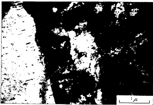
(b) Annealed at 760°C for 4hr; slab heated at 1250°C
