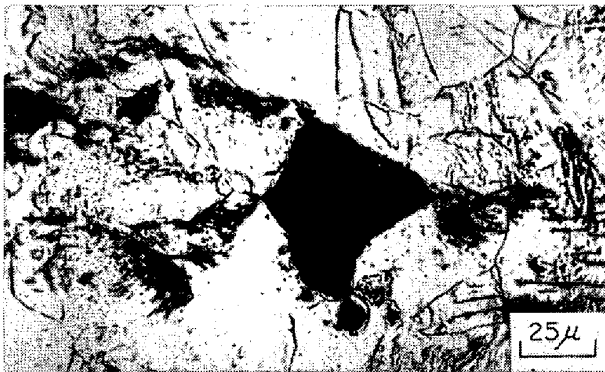
Photo. 3. Plastic deformation and microcracks initiated at an angular-type \text{Al}_2\text{O}_3 . P10B specimen (non-carburized). 2.3 \times 10^4 cycles to failure
