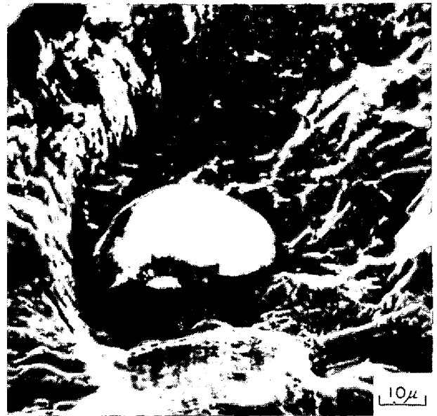
Photo. 9 Fractured surface of CP 5 A-2 specimen heat-treated after carburizing. 2.7 \times 10^6 cycles to failure. No outstanding change is observed around \text{Al}_2\text{O}_3 . (b) : enlarged a part of (a) (arrow).
