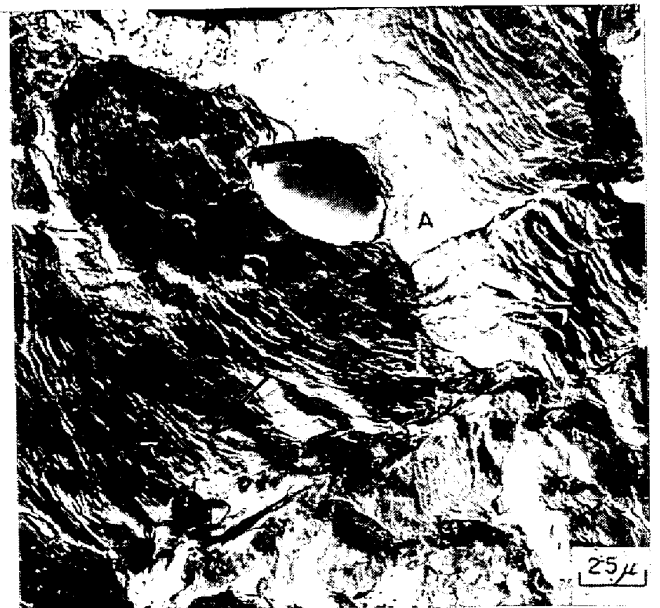
(b) The inclusion touches with grain boundary and crack propagation probably changes from transgranular to intergranular. 10% pre-strained A81 specimen. 1.4 \times 10^6 cycles to failure.
