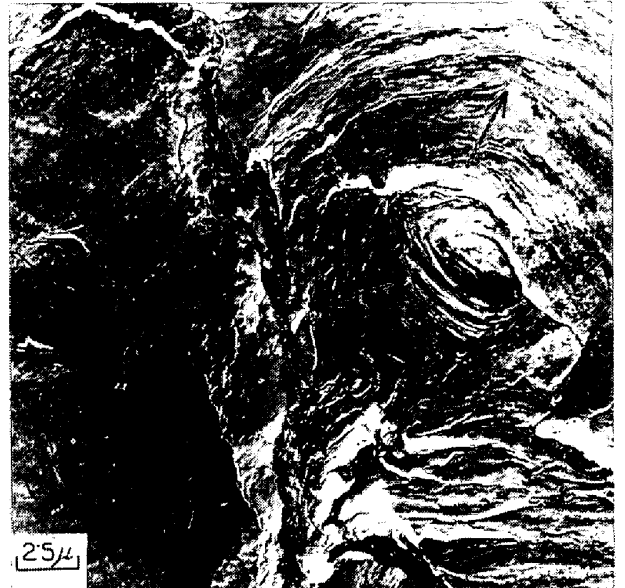
Photo. 15. Fatigue striations and inclusion in A73L specimen. Crack probably initiates from the inclusion before main crack reaches to the inclusion. 6 \times 10^4 cycles to failure.
