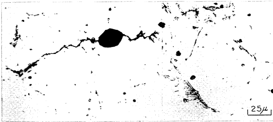
Photo. 8. Microcracks initiated from FeO type inclusion and those initiated from pre-grain boundary. C·OIL·A81 specimen. 0.6 \times 10^5 cycles to failure. No etched.
