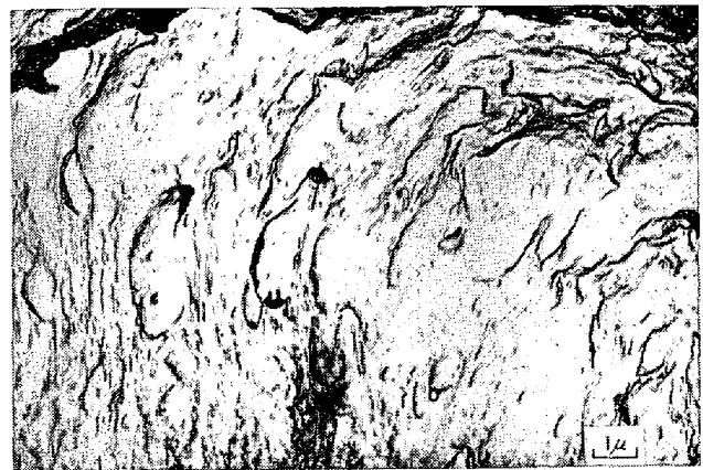
Photo. 7. A slip line of ferrite in machined surface layer (Electron micrograph in replica of specimen No 2). Workpiece speed 3m/ min, Depth of cut 70 \mu .
